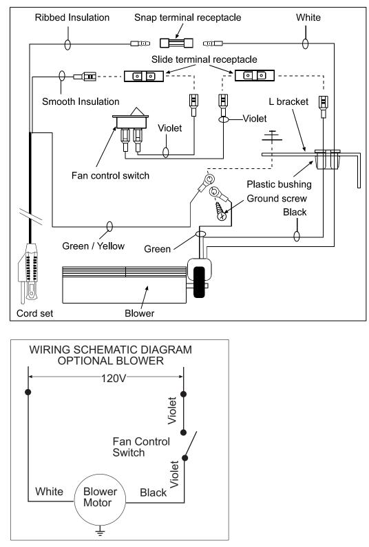
If any original wire, as supplied with this appliance, has to be replaced, it must be replaced with #18 gauge, 125°C, 2/64 insulation or its equivalent.
