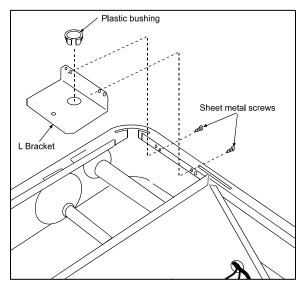
6. Lay down the blower beside the heater and pass the 3 wires through the plastic bushing.
